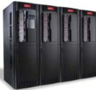
The Scalar i2000 features industry-leading density and a 19-inch rack form factor. One module holds up to 306 LTO tapes; four modules hold up to 1,674 tapes.
